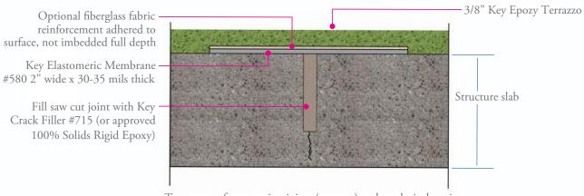
Treatment of contraction joints (sawcuts) and cracks is done in anticipation of horizontal movement.
